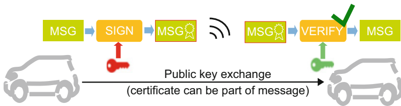
Fig. 2 Message authentication using digital signatures
