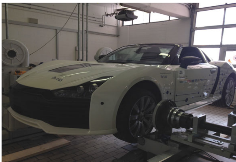
Fig. 10 The cars equipped with the RACE architecture. Top: physical appearance, bottom: car on test rig with direct coupling (all four wheels) to external electric motors that can induce very realistic driving dynamics scenarios
