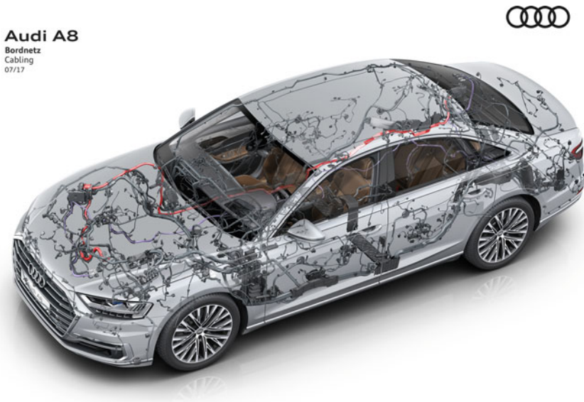
Fig. 1 The cabling topology of the 2018 Audi A8; note the actual ECUs are not shown
